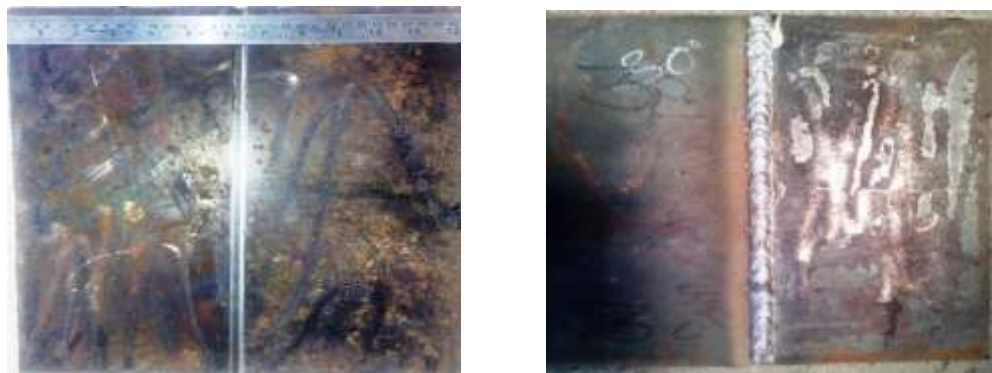
Figure - 4.6 Distortion Specimens Before and After Welding
