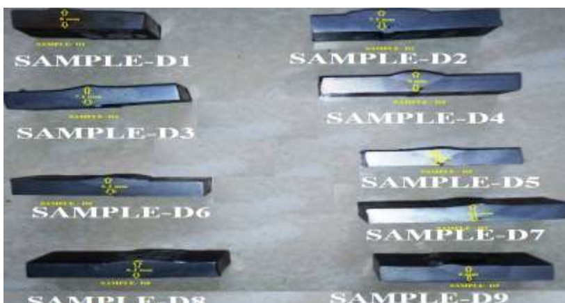
Figure - 4.6 Depth of Penetration Sample after Welding
