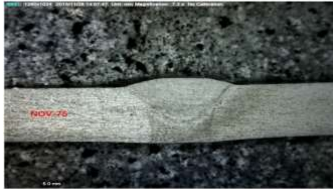
Figure - 4.5 Macro Test Inspections as Per Standard of ASTM
